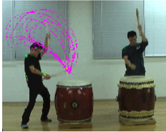
Fig.3-4-8 The trajectory of the right stick of Sub.A in the case of duo rhythmic performance with Sub.B
