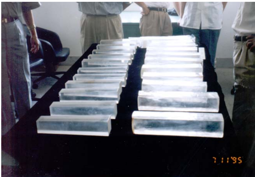
Figure A.1: Ingots of \text{CsI}(\text{Tl}) crystals produce by (a) Institute for Single Crystals in Ukraine and (b) Shanghai Institute of Ceramics. The Chinese crystals are grown by the Bridgman method. The Ukrainian crystals are produced by the Czochralski method. The growth speed of the crystal is \sim 1 mm/hour in either method.
