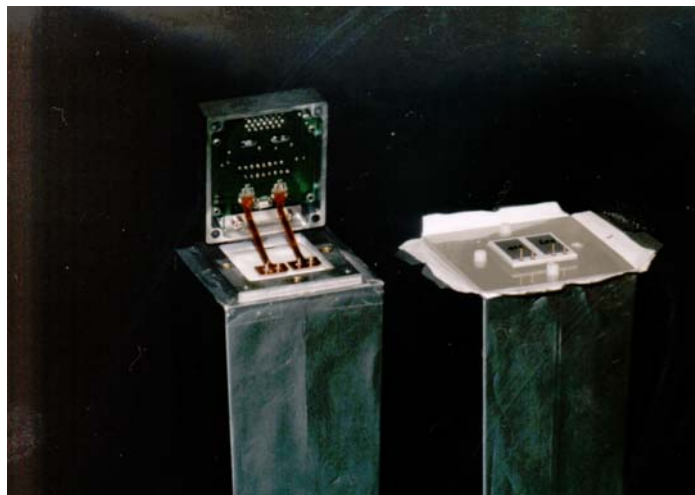
Figure 4.17: Assembly of CsI(Tl) counter module.
